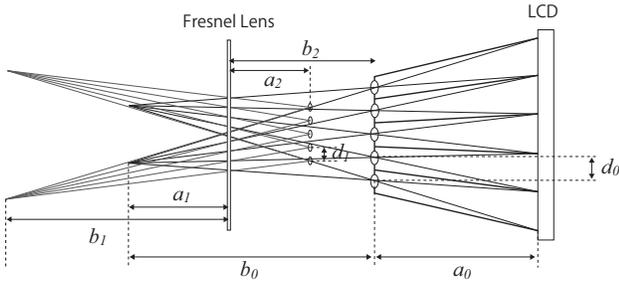
Figure 4: High-resolution optical system consisting of Fresnel lens.
