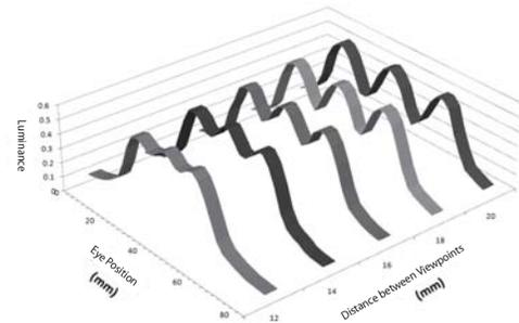
Figure 8: Luminance value as a function of spacing between projection lenses.
