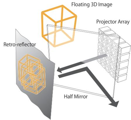
Figure 2: Basic principle of 3D display consisting of a projector array and a retro-reflector.
