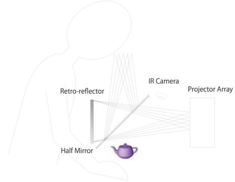
Figure 5: Two projection methods for superimposing 3D images in real space and IR-camera-based input interface.
