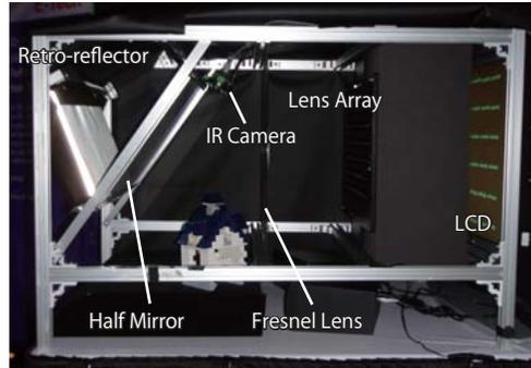
Figure 10: Prototype of the system.
