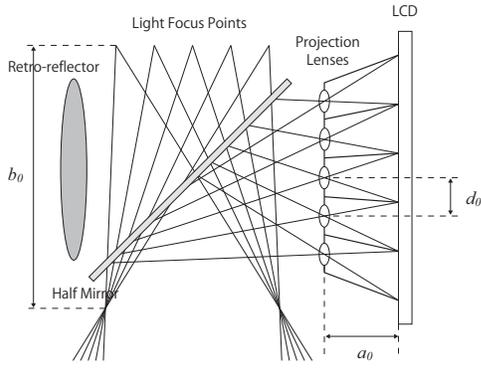
Figure 3: Optical system of the high-density projector array.
