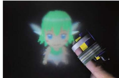
Figure 14: User touching the floating 3D character. Haptic feedback is provided to the user by the wearable haptic device.
