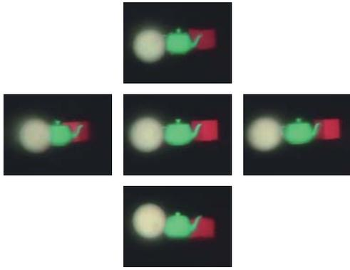
Figure 11: Projection of 3D object onto the retro-reflective screen as seen from multiple viewpoints.
