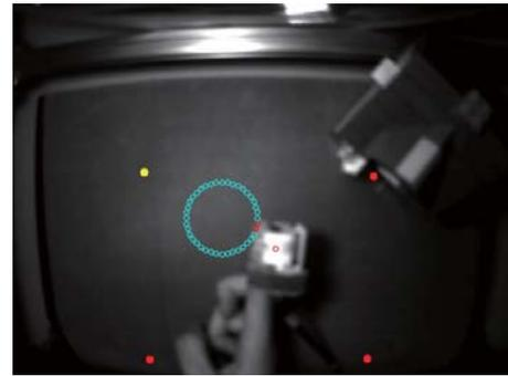
Figure 13: Result of image processing for detecting contact between the 3D image and the user's hand.
